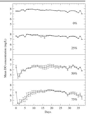
**Fig. 4** Mean daily dissolved oxygen (mg/L) concentrations for Year 1 in 0, 25, 50, and 75% fine sediment for egg burial depth at 10 cm. Error bars represent standard error. Dissolved oxygen (DO) dropped below 5 mg·L<sup>-1</sup> on days 2 and 3 for 50, and 75% fine sediment. DO was in acceptable ranges for all other days and treatments
