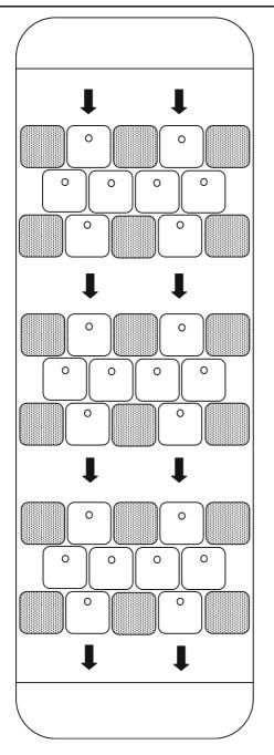
Fig. 2 Grid-like arrangement of incubation cells (white) and non-incubation cells (shaded) used to test the affects of fine sediment on survival of eggs to larval emergence robust redhorse. Circles represent standpipes used to monitor dissolved oxygen concentrations, which are upstream of egg pockets. Arrows denote direction of water flow
