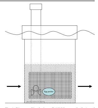
Fig. 1 Diagram of incubation cell (15.5 L square bucket) used to house gravel treatments and incubate robust redhorse eggs and larvae. The grid is the  $15 \times 10$  cm fiberglass mesh screen and the small dots represent the gravel mixture. The standpipe (3.2 cm diameter, 40 cm long) with holes (1.9 cm diameter) allowed dissolved oxygen concentrations to be monitored at depth of the egg pocket. Arrows denote direction of water flow
